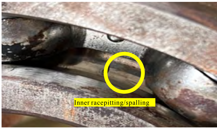
Figure 10. The physical condition of Pump Bearing #4 (Free End, 6321) after disassembly.
