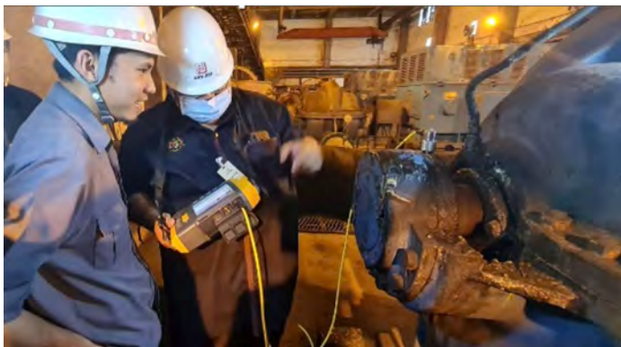
Figure 1: Tri-axial acceleration sensor mounted on bearing #4 (Free End, 6321) in vertical direction.
